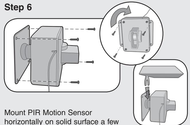
Mount PIR Motion Sensor horizontally on solid surface a few feet off the ground and within 900' of Base Station (rotate sensor to access screw holes). Unit should be able to swivel as needed. Attach sun/rain shield.
